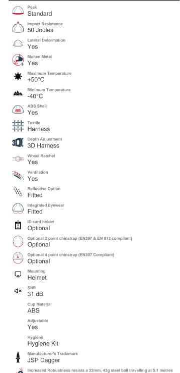
Increased Robustness resists a 22mm, 43g steel ball travelling at 5.1 metres per second. This is derived from the practical test which is to drop the ball (as stipulated) from a height of 1.3 metres.
