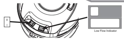
The vacuum cleaner is fitted with a low flow indicator. When the indicator is fully red, the air speed in the hose has dropped below 20m/s
